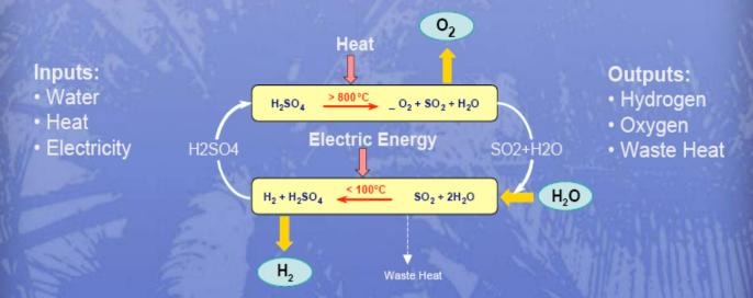
Two-step hybrid process; only sulfur-based chemistry
